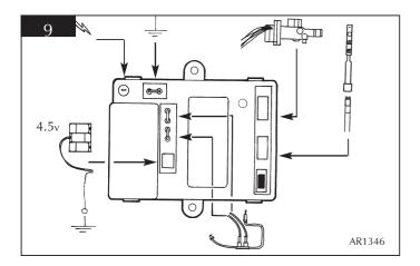
WHEN REPLACING WITH A NEW THERMOCOUPLE TAKE EXTREME CARE TO BEND THE NEW COMPONENT TO THE EXACT SHAPE AND TO KEEP THE CONNECTORS IN THE SAME ORIENTATION.
